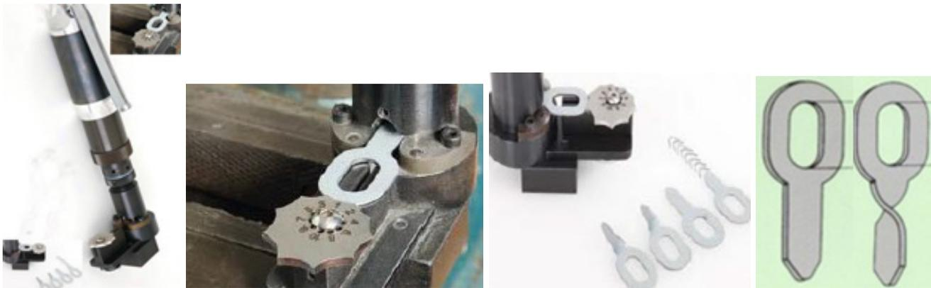
The pneumatic bit sharpener allows cutting the tip of pulling bits (pulling rings) in order to avoid complicated and tedious grinding of the bits one by one. Each bit can be sharpened up to 10 times.
